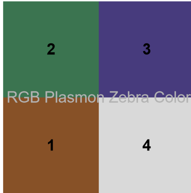
Рис. 7: Color of silver zebra with thickness 2h = 10 \text{ nm} , interstrip gap 2g = 40 \text{ nm} , that is deposited on glass substrate \varepsilon_e = 1 , \varepsilon_d = 2 ; 1, 2, 3 – color of PZ with strip width 2d = 200 \text{ nm} , 2d = 120 \text{ nm} , and 2d = 80 \text{ nm} , 4–bulk silver plate.
